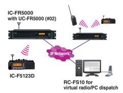
When using the IC-F5123D series in IDAS multi-site conventional mode, the IC-F5123D can communicate with other IDAS radio users working with other repeater sites and/or virtual radio/PC dispatch stations on the IDAS network.
