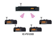
The IC-F5123D series allows you to call individual or group users. The radio automatically sends own ID number when the PTT button is held down. The alias name or individual/group ID is displayed on the LCD while receiving a message allowing you to identify who is calling.
