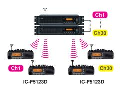
The IC-F5123D series can be used in an IDAS single-site trunking system.
