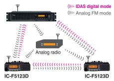
The IC-F5123D series can receive both analog mode and digital mode signals on a single channel and automatically selects the received mode to reply to the received call, while the talk back timer remains. It's a smart way to grow into digital radio – at your own pace, as your budget and comfort allow.
